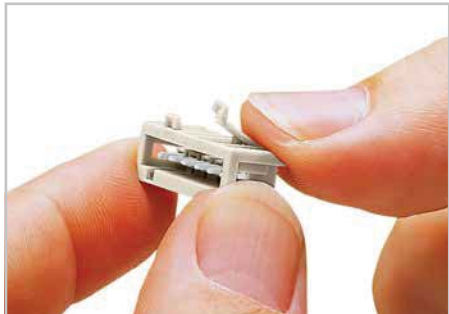
Coding a male header - fitting coding key(s).
